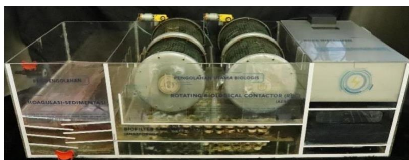
Gambar 1. Reaktor Pengolahan Limbah Cair Tekstil Berbasis Hybrid Attached Growth Biofilm Terintegrasi Arduino (Rahmadi et al. (2022)).
